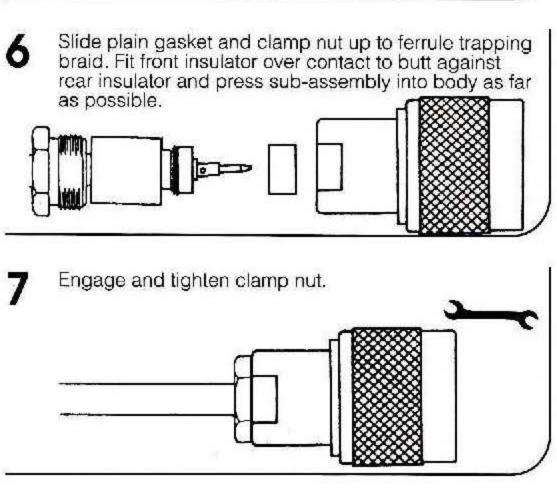
Note: a plug body is shown, but these instructions arc relevant to both plugs and jacks. The characteristics of the contacts and insulators may vary from the drawings shown.
